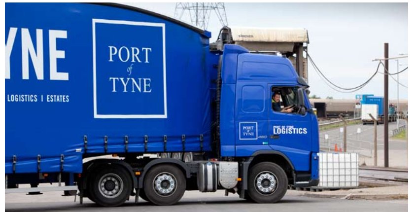
FANCY FLEET/ THE PORT OF TYNE TRUCKS ARE GETTING GREENER WITH NEW AERODYNAMIC TRAILERS, MORE FUEL EFFICIENT TYRES & AUTOMATIC IDLING CUT OFF
